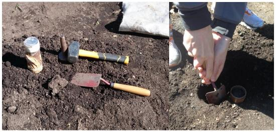
Figure 9. Collection equipment and techniques of soil sampling
