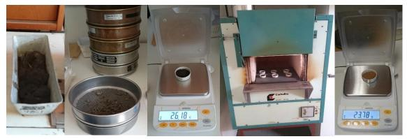
Figure 17. Weighing of samples before and after before and after the combustion process
