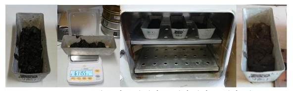
Figure 16. Weighing of samples before and after before and after drying
